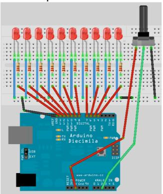
This is the same circuit as in Project 5, but we have simply added the potentiometer and connected it to 5v, Ground and Analog Pin 5.
