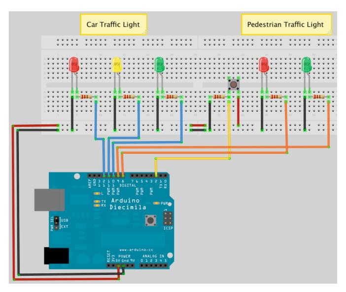
This time we are going to extend the previous project to include a set of pedestrian lights and a pedestrian push button to request to cross the road. The Arduino will react when the button is pressed by changing the state of the lights to make the cars stop and allow the pedestrian to cross safely.
