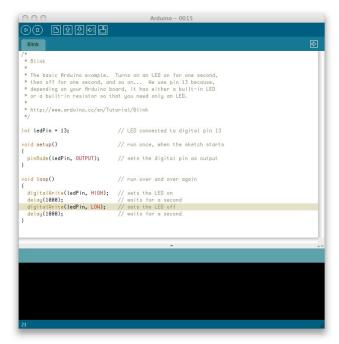
Now that your Freeduino has been connected and the drivers for the USB chip have been installed, we are now ready to try out the Arduino for the first time and upload your first Sketch.
