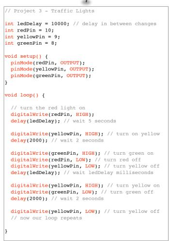
In the next project, we are going add to this project by including a set of pedestrian lights and adding a push button to make the lights interactive.
