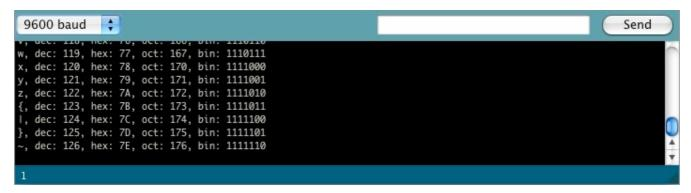
To the right of this is a blank text box for you to enter text to send back to the Arduino and a **Send** button to send the text within that field. Note that no serial data can be received by the Serial Monitor unless you have set up the code inside your sketch to do so. Similarly, the Arduino will not receive any data sent unless you have coded it to do so.
