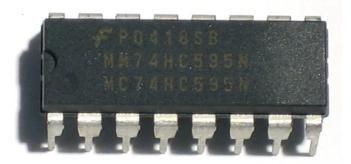
As the outputs are simply ON's and OFF's of an output voltage, they can also be used to switch other low powered (or even high powered devices with the use of transistors or relays) devices on and off or to send data to devices (e.g. An old dot matrix printer or other serial device).
