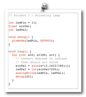
Verify and upload. You will now see your LED pulsate on and off steadily. Instead of a simple on/off state we are now adjusting it's brightness. Let's find out how this works.
